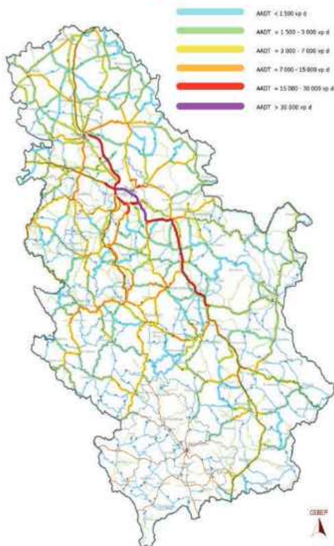
Figure 2. The value of Average Annual Daily Traffic on the road network of Serbia
